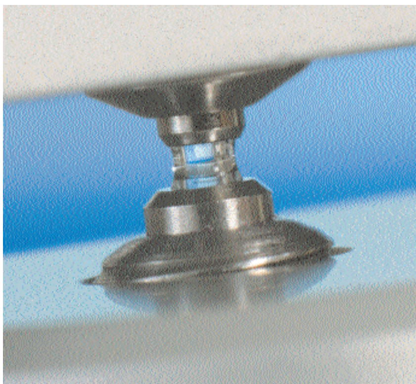
Figure 3b. 1 \mu l sample 'bridging' the optical fibers.
