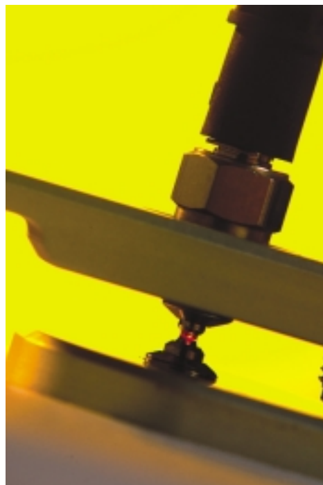
Figure 2 When the sample apparatus is closed, the upper measurement pedestal slightly compresses the droplet and then a sample column is drawn. Surface tension alone holds the sample in place.
