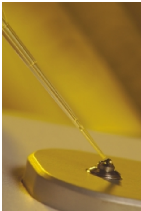
Figure 1 With the sampling apparatus open, a droplet of sample is pipetted onto the lower measurement pedestal.
