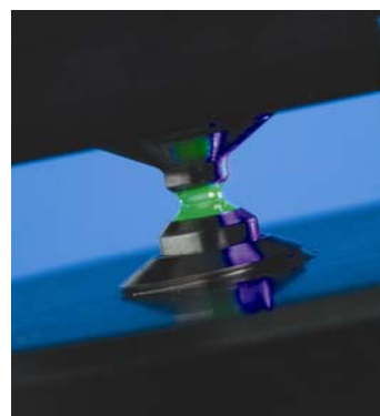
Figure 1: Close up view of the sample retention system of the NanoDrop 3300 with a concentrated sample of FITC forming a column between the measurement pedestals.
