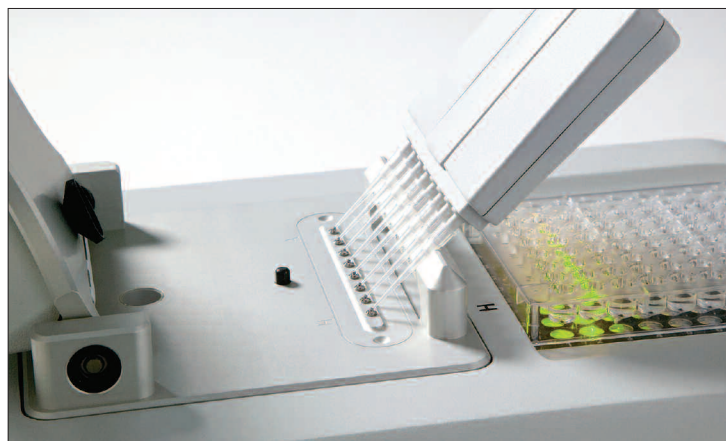
Figure 1. The sample-retention system of the NanoDrop 8000 uses surface tension to hold and measure up to eight 1 µL protein samples at a time.
