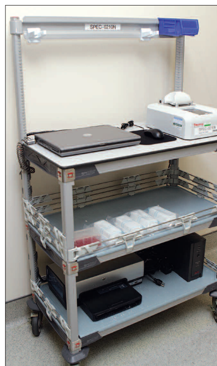
Figure 2. The NanoDrop 8000 is used on a movable cart for UV-Vis analysis in real time in Diosynth Biotechnology’s protein-production facility.
